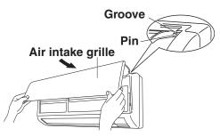
To attach the air intake grille to the indoor unit, press its bottom right and left corners as well as its bottom center into place.
